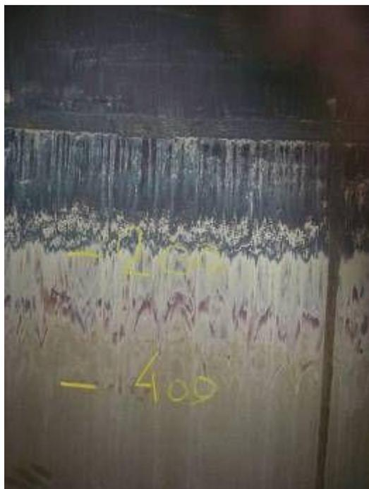
The cross cut ends of the tray support clips did also not show any corrosion, the marks from the fabrication were still clearly visible; the conclusion was that the Safurex<sup>®</sup> is in such a condition as it was never exposed to any carbamate solutions.
