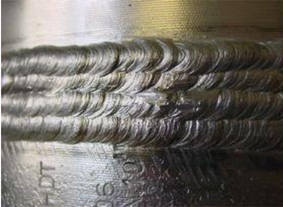
**Photo 14: Safurex<sup>®</sup> rootrun in HP Piping**
