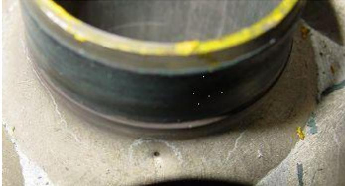
The wall thickness of the heat exchanger tubes in the HP Stripper was measured. Since there was no base line measurements done it was not possible to determine a corrosion rate, however what can be concluded is that the wall thickness of the heat exchanger tubes is still within the tolerances of the new tubes.
