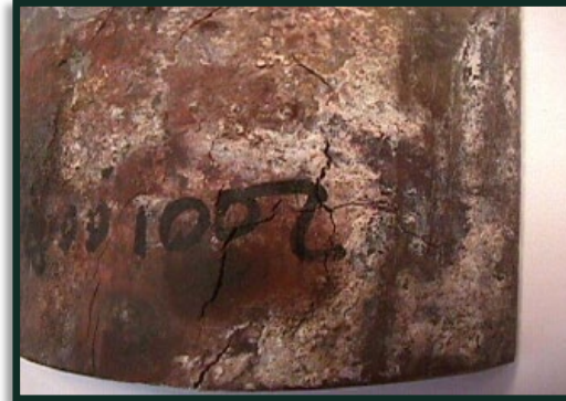
C-steel clamp allowing ingress of water and serious chloride SCC in AISI 304L pipeline underneath the clamp
