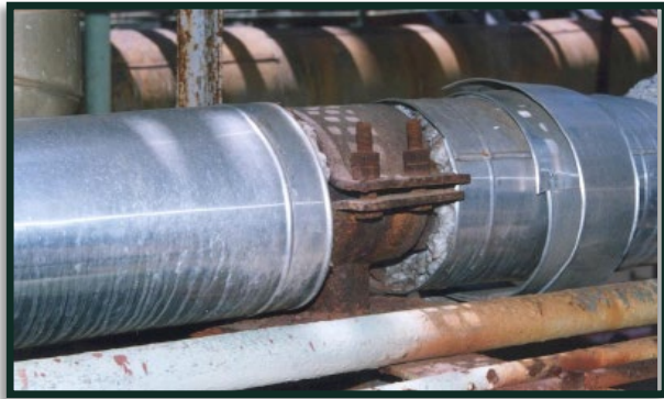
C-steel clamp allowing ingress of water and serious chloride SCC in AISI 304L pipeline underneath the clamp
