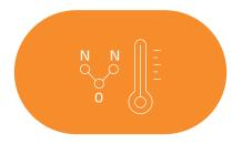
High tail gas temperature boosts N2O decomposition without adding external agents like natural gas.
