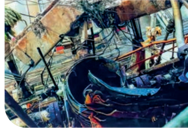
Ruptured HP Scrubber
