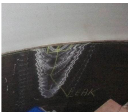
Figure 3: Leak found in the circumferential weld between the X2CrNiMo25-22-2 relined part (top) and original 316LUG liner
