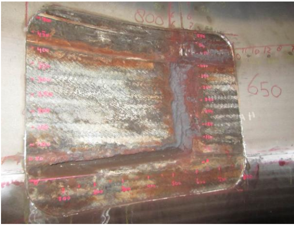
Figure 4: Corrosion of the c-steel pressure shell visible
