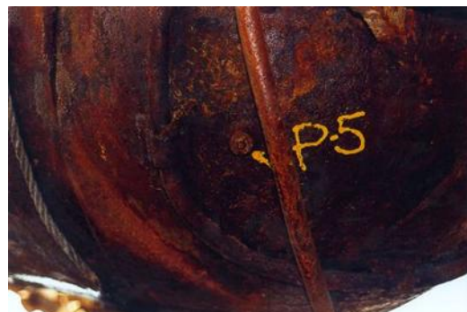
Figure8: hemi-head part of dome with plugged LDS hole
