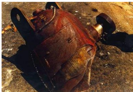
Figure8: hemi-head part of dome with plugged LDS hole
