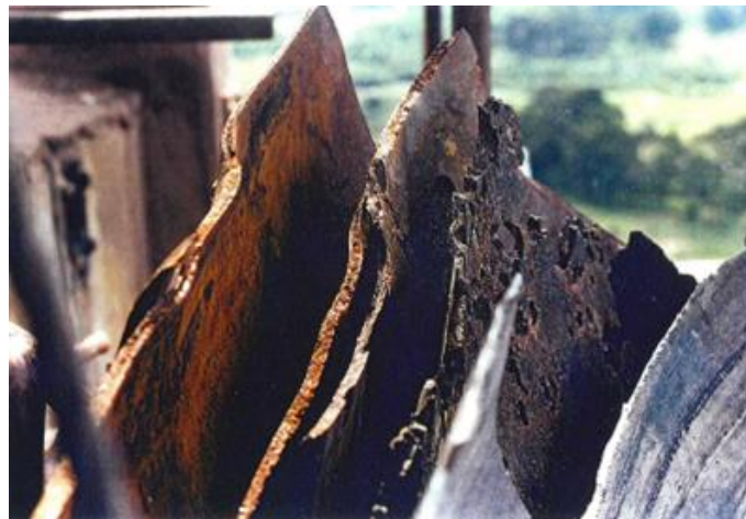
Figure 5: Severe corrosion of three inner c-steel layers
