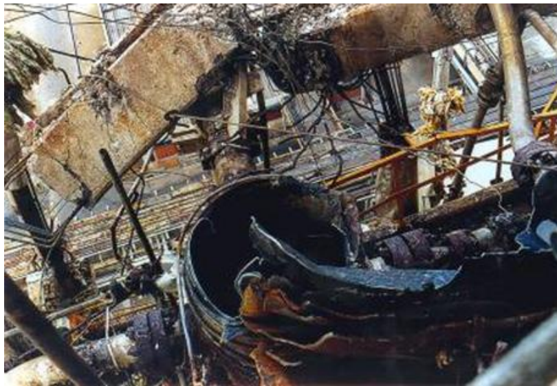
Figure 3: Damaged top part of HP Scrubber and
