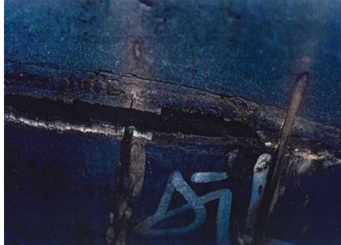
Figure 7: Leak path via fillet weld of cover plate and leak detection hole towards the multi-layered pressure shell.
