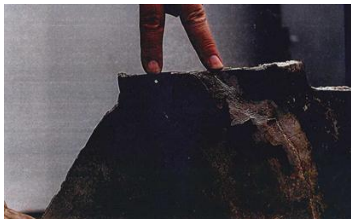
Figure 6: Backside of liner plate with carbamate corrosion
