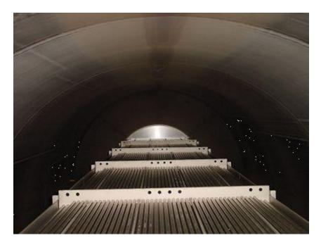
In the HP Stripper a pinhole in a tube-to-tubesheet welding was found in the top tubesheet. With different materials this would have led to active corrosion and even a leaking tube-to-tubesheet weld could not be excluded. This pinhole however did not show any active corrosion.
