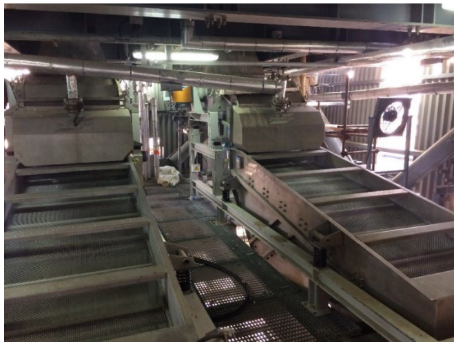
Fig. 6: Lump screens installed in the granulation plant
