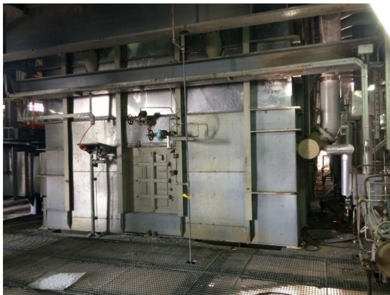
Fig. 4: Side picture of the installed granulator in the granulation plant
