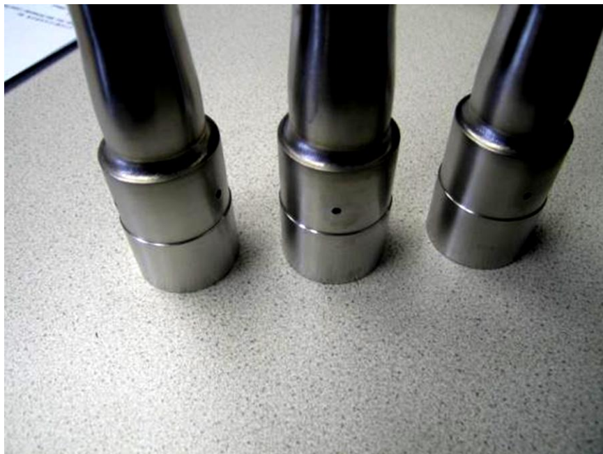
Safurex ® Degree liquid divider produced and installed in HP stripper.
