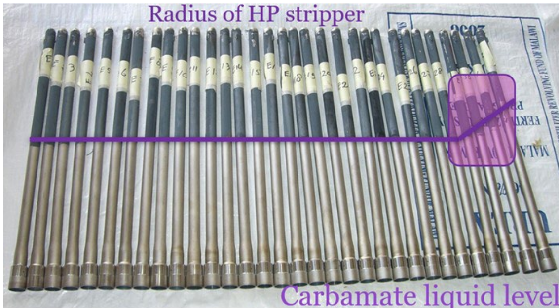
Fig. 5: Carbamate liquid level noticed in the liquid dividers when ordered according to their location over the HP Stripper radius. Level at the outer side is larger.
