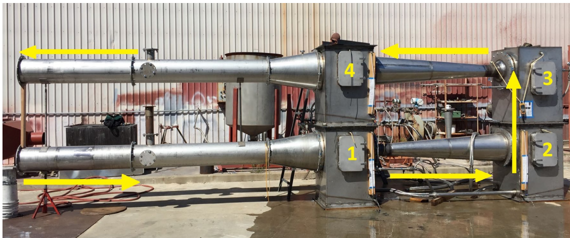
Fig. 14. The pilot unit during fabrication at the ECI workshop with indicated boxes and airflow direction
