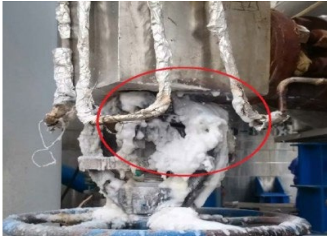
Figure 10: Leaks along a threaded bonnet connection of a high-pressure drain valve.
