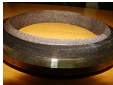
Figure 3 and 4: Line sealing principle of a lens ring (left) and a real life example showing normal passive corrosion on the process side of the lens ring (right)
